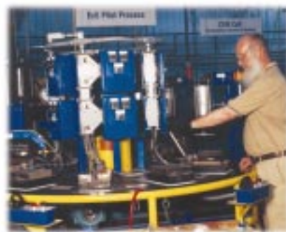
Molds filled with EcE compound are loaded and unloaded during the curing cycle by a ten-station rotary press custom designed for a more flexible and cost-effective process.
