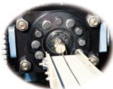
Extrusion presses produce a multitude of conductive elastomer profiles in 40 different compounds which are used in both military and commercial applications.
