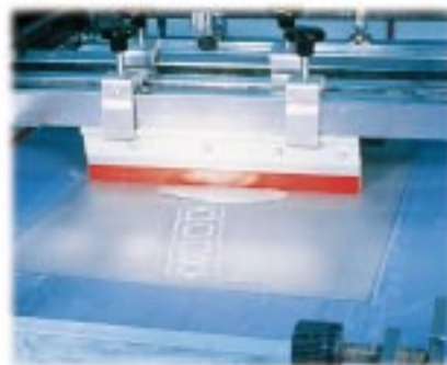
Screen printing conductive elastomer compounds onto metal or metalized plastic panels provides a low profile, intricate shaped EMI gasket while bonding securely to the panel surface.
