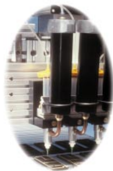
Computerized XYZ form-in-place dispensing machines deposit conductive elastomer compounds onto miniaturized thin wall multicompart housing covers.
